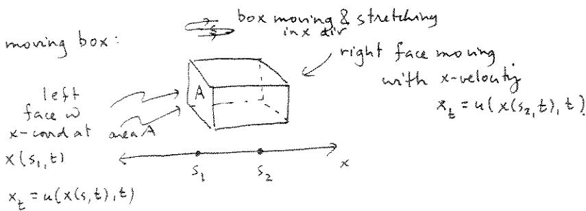
Newton:  $\frac{d}{dt} (\text{momentum in fluid box}) = \text{net forces.}$
