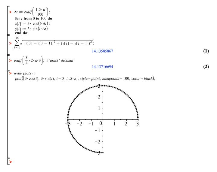
How to compute curve lengths with Calculus:
