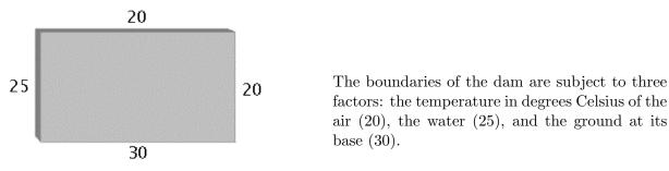
An analysis of the heat transfer from the three sources will be done from the equilibrium temperature, which is found by the Mean Value Property below.
