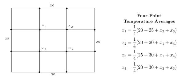
Solve the equations for the four temperatures  $x_1 = 23.125, x_2 = 21.875, x_3 = 25.625, x_4 = 24.375$ by any method.
