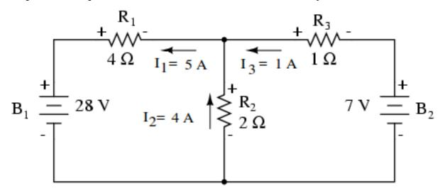
The **Branch Current Method** can be used to find a  $3 \times 3$  linear system for the **branch currents**  $I_1, I_2, I_3$ .
